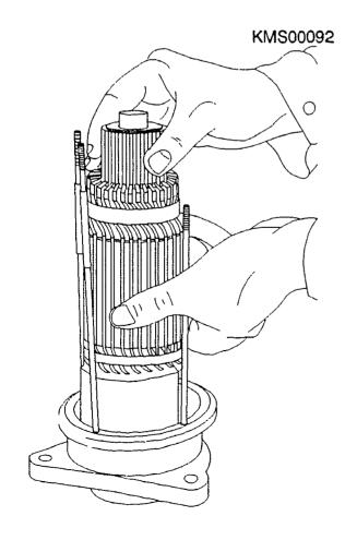
STARTING-MOTOR ASSEMBLY Assembling drive-end bearing Clamp stator frame in clamping support. Carefully insert drive-end bearing complete with armature in stator frame. Pay attention to marking. The stud bolts must not damage the field windings. Clamping support: 0 986 619 362
